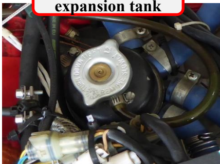
Coolant expansion tank
